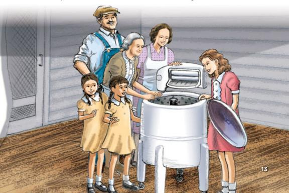
The next Monday, Wendy's mother tried out the new machine. She filled the machine with water, put the washing in, and sprinkled the soap flakes on top. When she turned it on, the machine shuddered into action. The paddle-like agitator was powered by electricity, which meant no one had to stir with the paddle.
