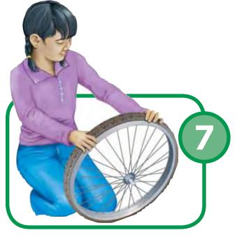
Use the bike pump to blow the tire up. The tire should feel firm to the touch. Then put the wheel back on the bicycle frame.
