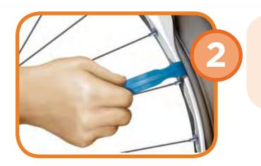
Pick up a tire lever. Place the thin end of the lever between the tire and the rim of the wheel.
