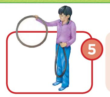
Check the tire for the cause of the flat. Carefully remove any objects. Use your bike pump to put just a little air in your new tube. Put the tube into your old tire. Be sure it doesn't have any twists or kinks.
