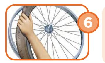
Find the hole in the rim of your wheel for the tire valve. Put the tire valve in the tube through the hole as you pull the tire and tube over the wheel. Use your fingers to ease the tire onto the wheel.
