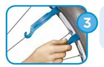
Do the same thing with the other two tire levers. Find a spot on the wheel about two spokes over from where you placed the first tire lever.
