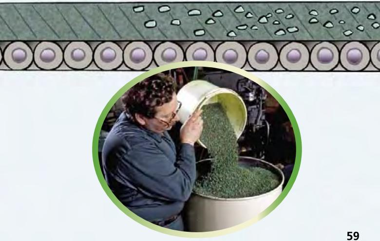
Next the plastic bits are melted until they are soft. The soft plastic can be used to make many new things.
