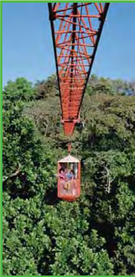
A canopy crane lowers researchers from the Smithsonian Tropical Research Institute into the canopy of a rain forest in Panama.
